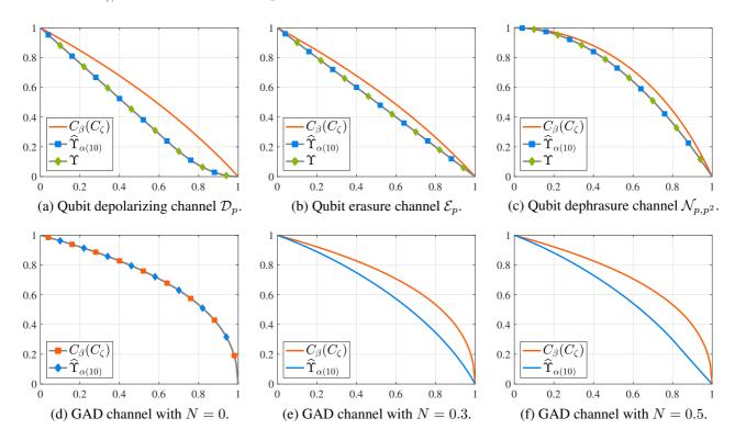
Figure 10: Comparison of the strong converse bounds on the classical capacity for the qubit depolarizing channel  $\mathcal{D}_p$ , the qubit erasure channel  $\mathcal{E}_p$ , the qubit dephrasure channel  $\mathcal{N}_{p,q}$  with  $q = p^2$ , and the generalized amplitude damping channels  $\mathcal{A}_{p,N}$  with different parameters. Note that  $C_\beta$  and  $C_\zeta$  coincide for all these examples. The horizontal axis takes value of  $p \in [0, 1]$ .
