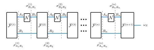
Figure 12: A schematic diagram for the magic state generation protocol that uses a quantum channel n times. Every channel use is interleaved by a free CPWP operation  $\mathcal{F}^{(i)}$ . The goal of such a protocol is to produce an approximate magic state  $\omega_S$  in the end.
