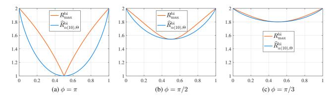
Figure 7: Comparison of the strong converse bounds on the two-way assisted quantum capacity of the bidirectional channels in (104) with the dephasing parameter choosing from  $\phi \in \{\pi, \pi/2, \pi/3\}$ . The horizontal axis takes value of  $p \in [0, 1]$ .
