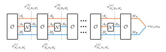
Figure 3: A schematic diagram for the protocol of  $\mathcal{O}$ -assisted quantum communication that uses a quantum channel *n* times, where  $\mathcal{O}$  is usually chosen as LOCC or PPT. Every channel use is interleaved by an operation in the class  $\mathcal{O}$ . The goal of such a protocol is to produce an approximate maximally entangled state  $\omega_{M_AM_B}$  between Alice and Bob. The systems in red are held by Alice while the systems in blue are held by Bob.
