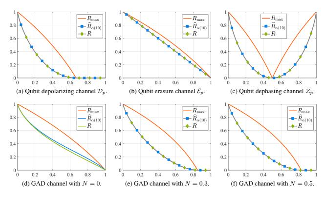
Figure 5: Comparison of the strong converse bounds on the unassisted quantum capacity of the qubit depolaring channel  $\mathcal{D}_p$ , the qubit erasure channel  $\mathcal{E}_p$ , the qubit dephasing channel  $\mathcal{Z}_p$  and the generalized amplitude damping channels  $\mathcal{A}_{p,N}$ . The horizontal axis takes value of  $p \in [0, 1]$ .
